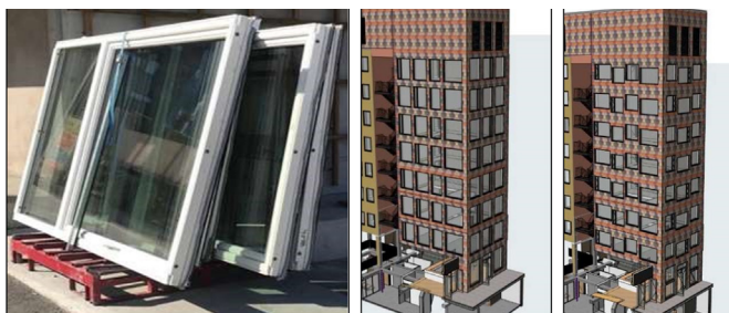
The windows were removed from a housing project in Kværnerbyen. Photo: Resirgel Extension façade, designed with 1) new windows, 2) used windows. Illustrations: Mad Arkitekter
