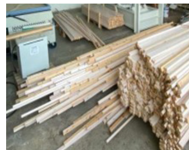
Wooden slats dismantled from the ceiling in the corridors of Refstad school. Photo: Anne S Nordby Storage and production at LUN. Photo: Lars Ulrich Nielson
