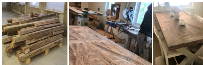
Surplus after demolition: A stack of structural timber transformed into beautiful tables. Photo: Driftwood
