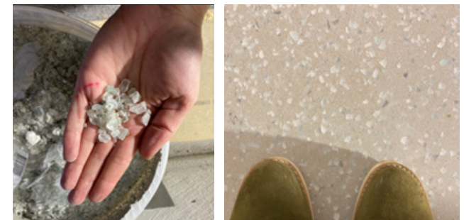
Glass concrete: Concrete floor with recycled façade glass.
